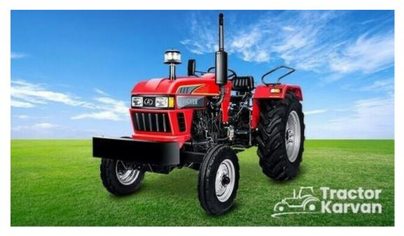
**Engine & Performance**- Eicher 485 HP has 45 horsepower. This tractor's engine capacity is 2945 cc; the cubic capacity influences the power provided by the engine. It has three cylinders and an air-cooled cooling system.
